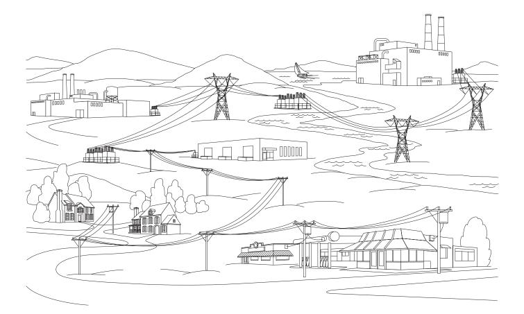
There are several sources used to produce power. Coal, oil, and uranium are fuels used to convert water into steam which in turn drives a turbine. Some utilities also use gas turbines, or both gas and steam turbines, for combined cycle operation. The output shaft of the turbine is connected to an AC generator. The AC generator is rotated by the turbine. It is the AC generator which converts the mechanical energy into electrical energy.
