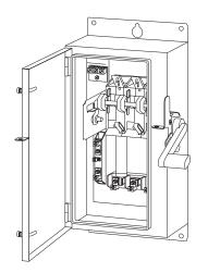
A case or housing. Guidelines for various types of electrical enclosures are provided by the <u>National Electrical</u> <u>Manufacturers Association (NEMA)</u>.
