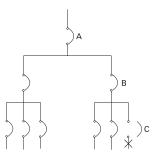
A control device with two or more positions used to manually open and close contacts.
