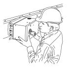
A prefabricated electrical distribution system that uses *bus bars* in its own protective *enclosure*.
