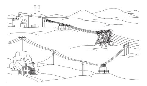
The most common supply system used in residential applications today is a single-phase, three-wire supply system. In this system, there are 120 volts between either hot wire and neutral and 240 volts between the two hot wires. The 120-volt supply is used for general-purpose receptacles and lighting. The 240 volt supply is used for heating, cooling, cooking, and other high-demand loads.
