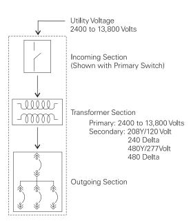
A primary switch is used to provide a means to connect and disconnect the secondary unit substation from the supply service. The transformer section can be liquid filled, ventilated dry type, or a cast-coil type. The outgoing section can be a Siemens Sentron switchboard, such as the RCIII, or Type R lowvoltage switchgear.
